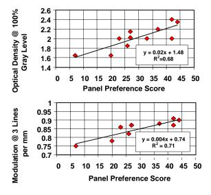
Figure 8 Modulation and Optical Density vs. Subjective Scores
