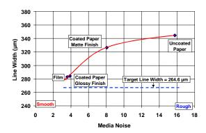
Figure 4 Effect of Media on Line Width
