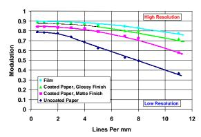
Figure 5 Effect of Media on Modulation (Resolution)
